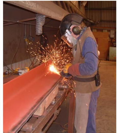
Zirc + in Action preparing sections for welding
