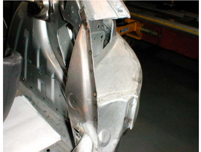
Flanges (Rear Boot) Cleaning all flange surfaces
