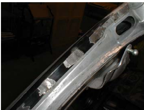
Rear Boot Aperture - Dressing 'plug' welds
